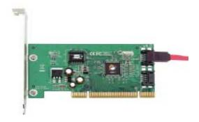
Figure 3. Connecting the Serial ATA data cable
